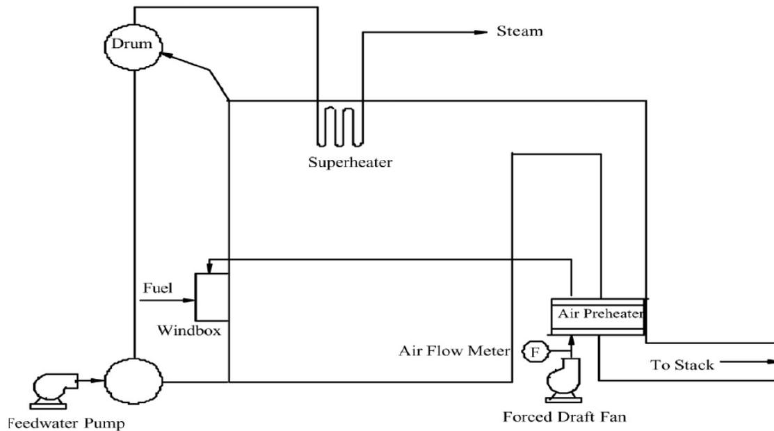
Fig. 4: Figure 7-4. Schematic Diagram of Boiler 9
