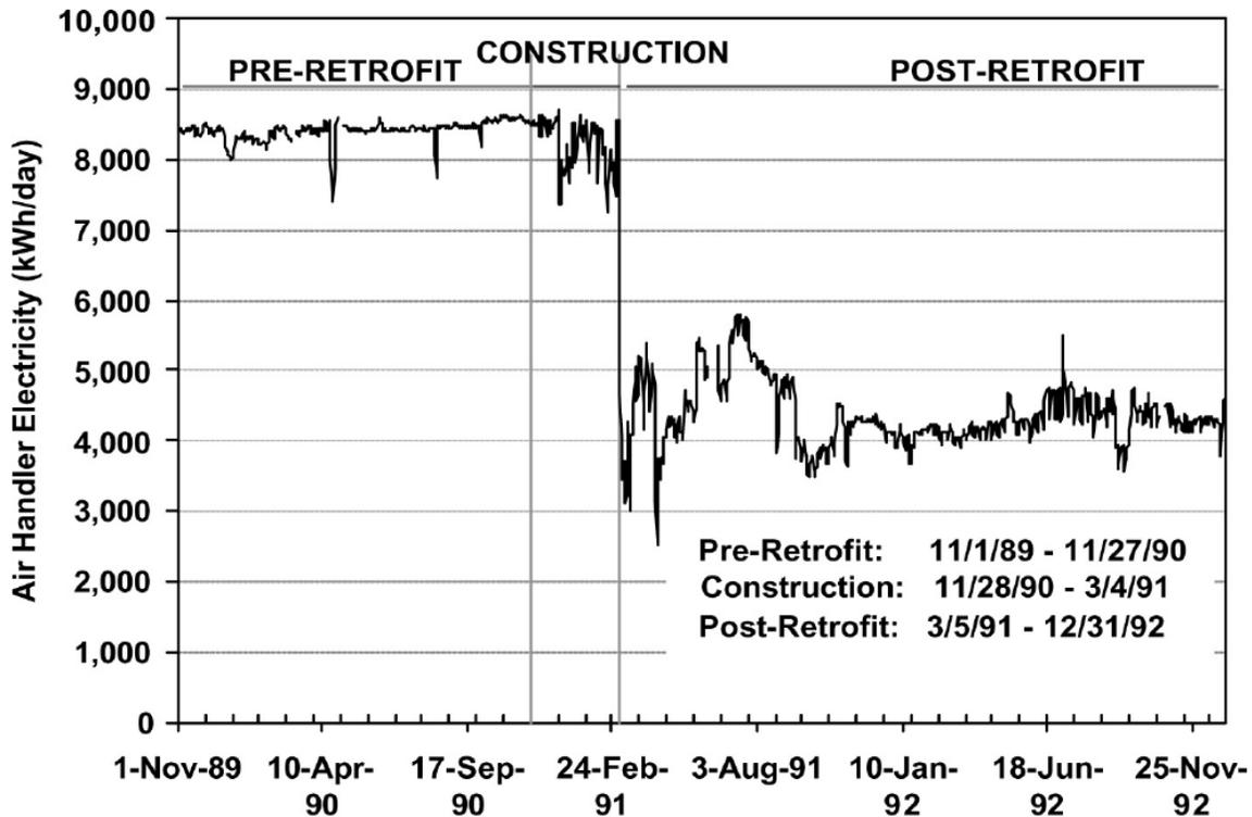
Fig. 1: Figure 9-1. Daily Electricity Consumption for Approximately One Year Before a Retrofit and Two Years After the Retrofit
