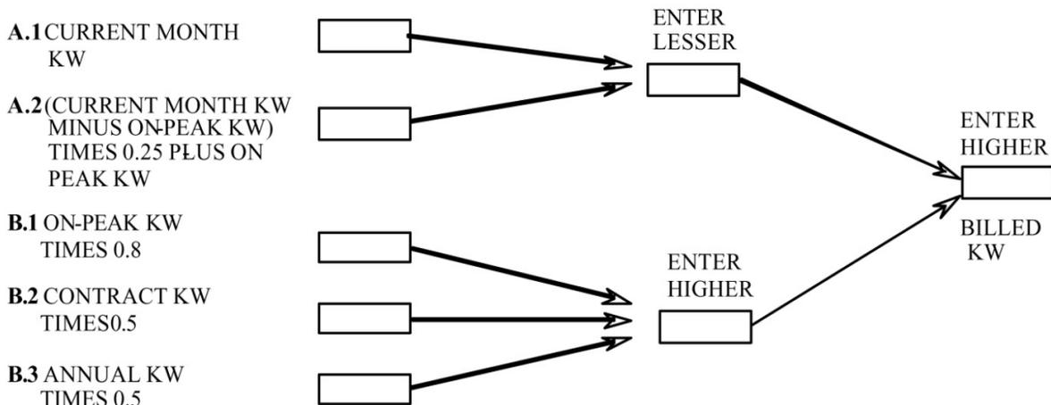
Fig. 7: Figure 8-7. Flowchart for the Calculation of Monthly Billing Demand
