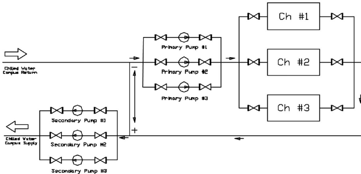
Fig. 11: Figure 5-11. Primary and Secondary Loop Configurations for the South Satellite Plant on the Texas A&M Campus
