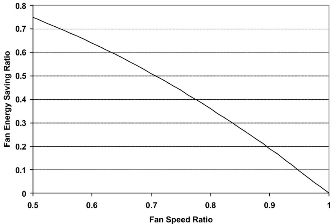
Fig. 4: Figure 3-4. Potential Fan Energy Savings Using Fan Speed Limiting
