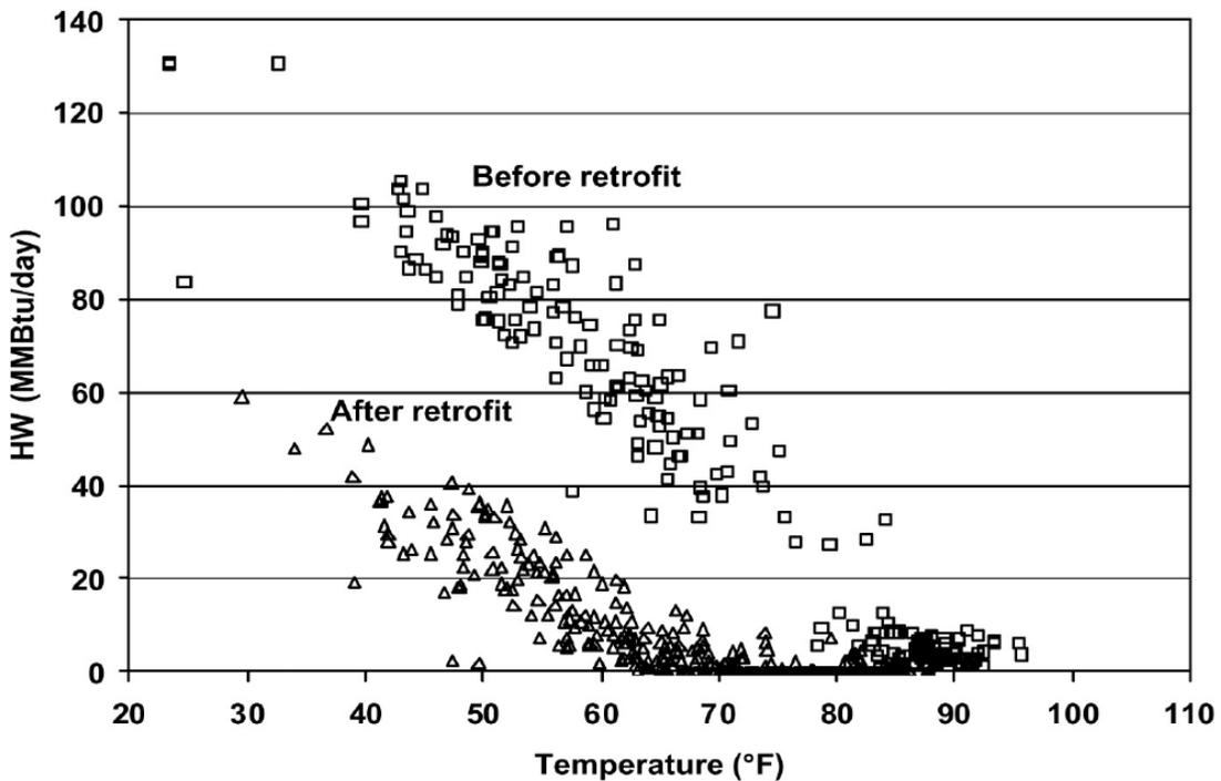
Fig. 4: Figure A-4. ZEC Daily Hot Water Consumption in 1990 Before the Retrofit and in 1994 After the Retrofit
