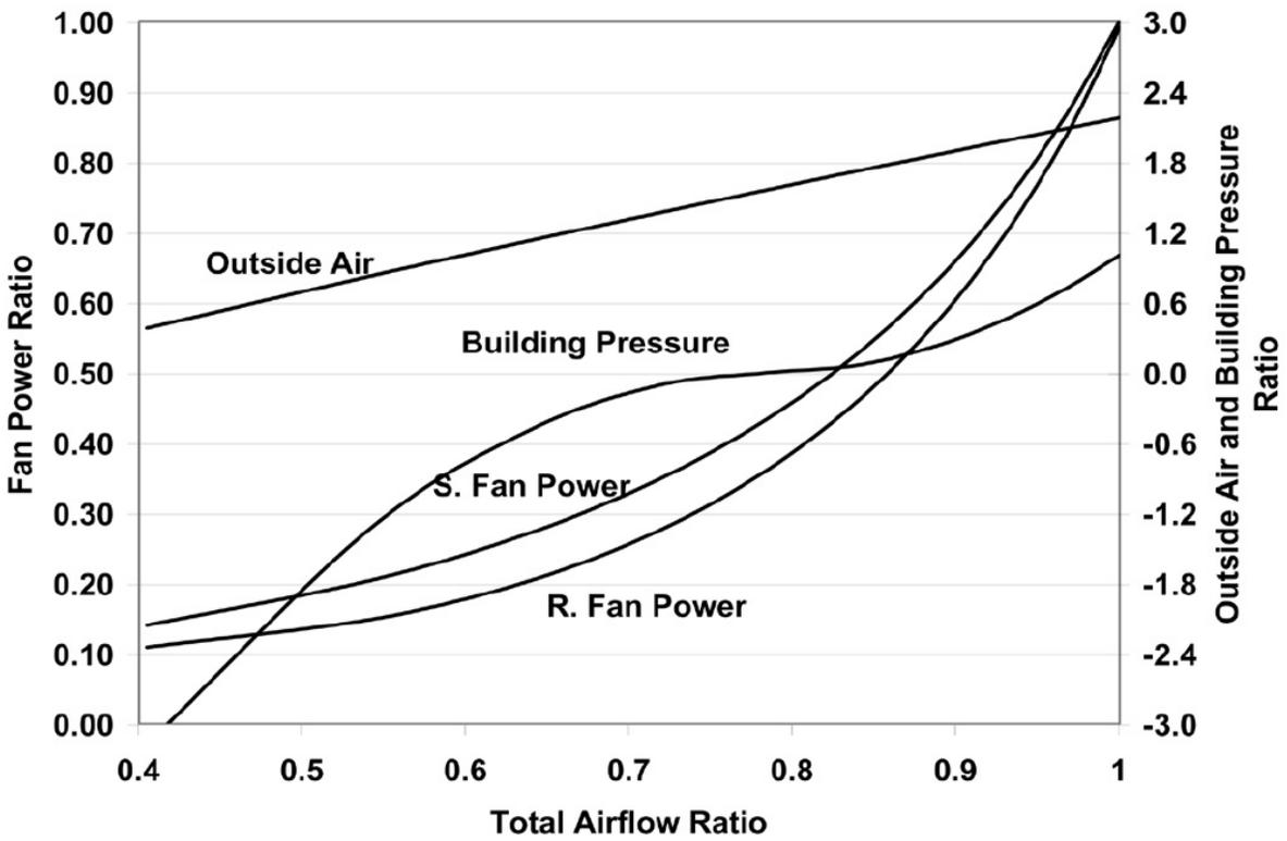
Fig. 22: Figure 4-22. Simulated Building Pressure, Outside Air Intake and Fan Power Using Typical Fan Tracking Control
