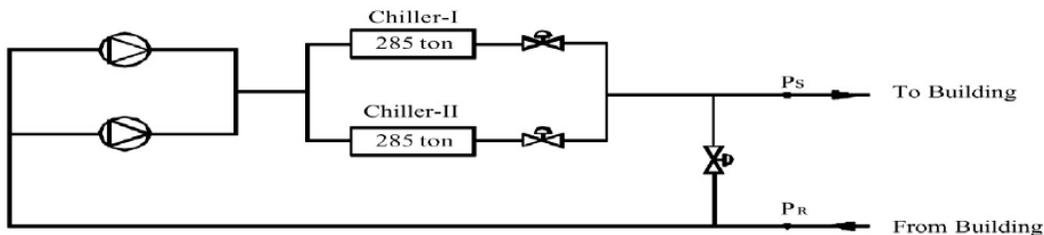
Fig. 9: Figure 5-9. Schematic Diagram of Chiller Plant at MRI Building
