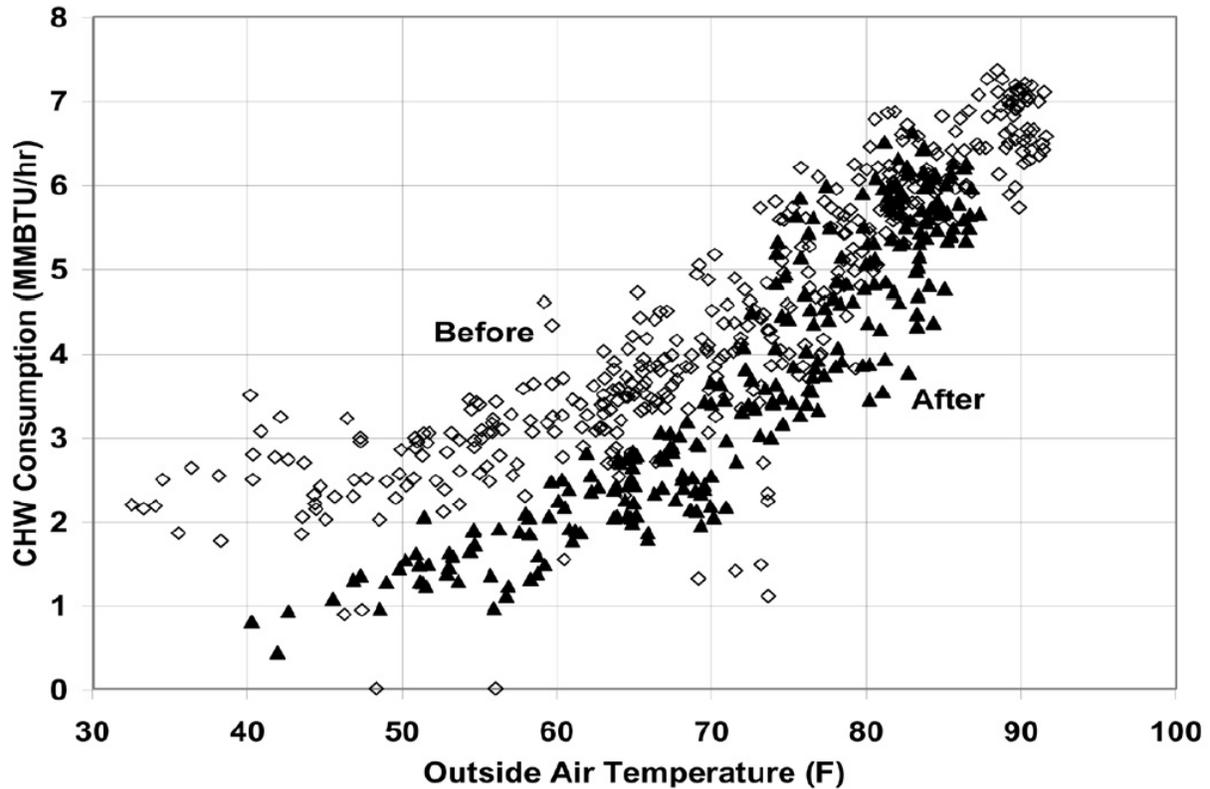
Fig. 7: Figure 4-7. Comparison of Measured Daily Average Chilled Water Consumption Before and After Implementation of the Optimal Hot and Cold Deck Temperature Reset Schedules
