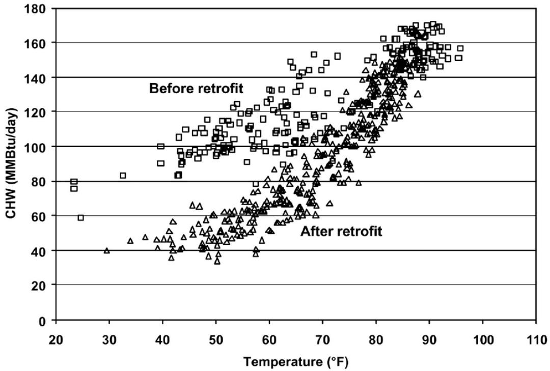
Fig. 3: Figure A-3. ZEC Daily Chilled Water Consumption in 1990 Before the Retrofit and in 1994 After the Retrofit
