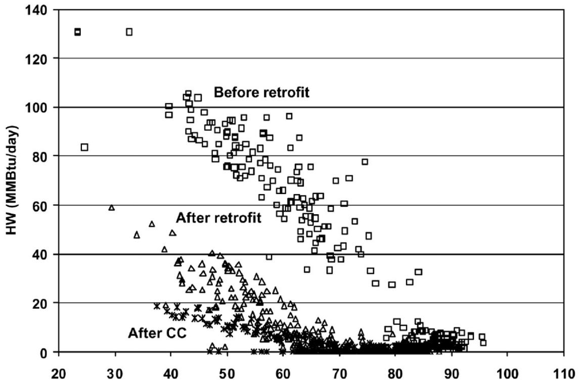
Fig. 7: Figure A-7. ZEC Daily Hot Water Consumption for 1990 Before the Retrofit, 1994 After the Retrofit and 1997 After CCSM
