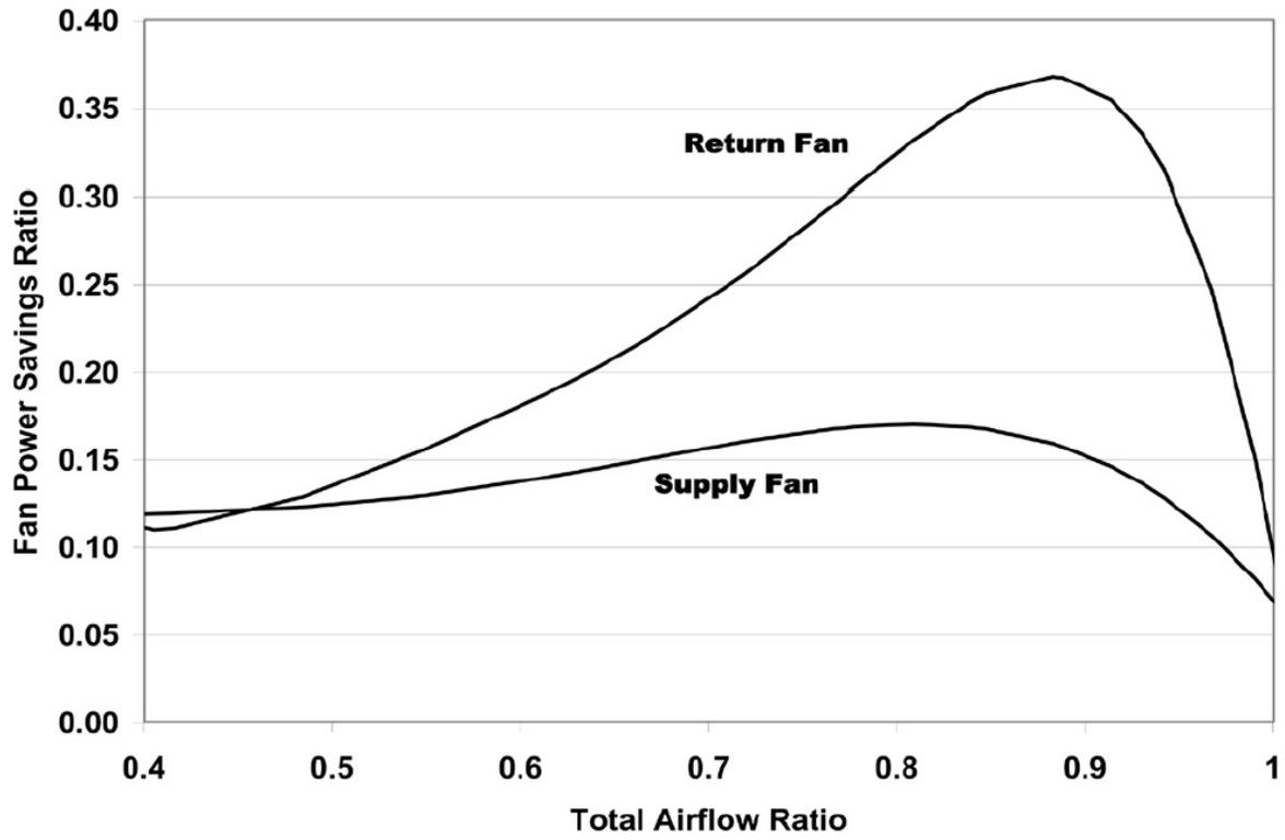
Fig. 24: Figure 4-24. Potential Fan Power Savings of the VSDVT Method
