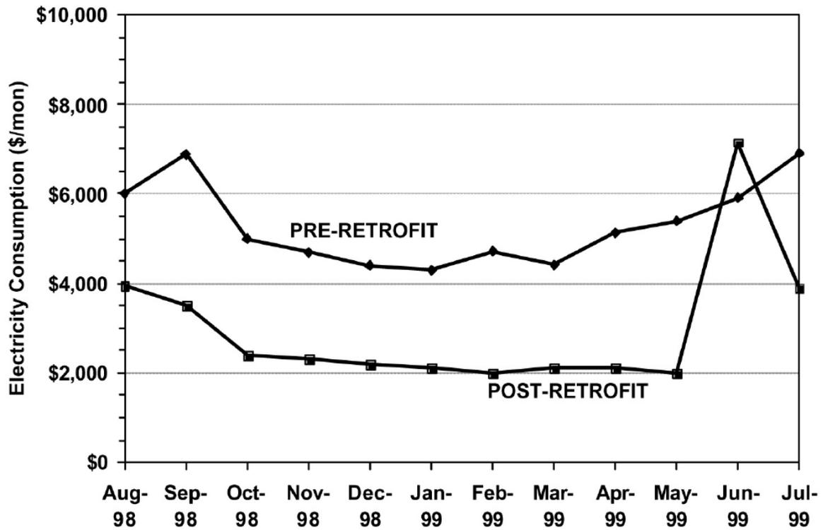
Fig. 2: Figure 9-2. Comparison of Monthly Utility Bills Before (Top Line) and After (Bottom Line) a Retrofit
