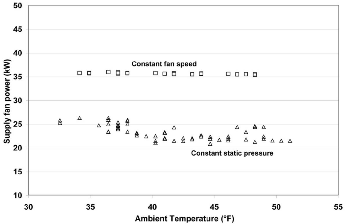
Fig. 20: Figure 4-20. Measured Hourly Supply Air Fan Power for Both the CSFS and VSFS Operations
