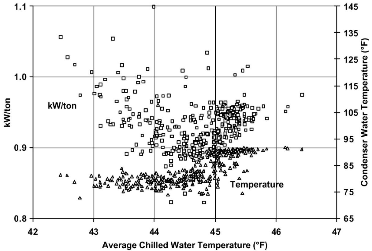
Fig. 1: Figure 6-1. Measured Chiller Plant Efficiency and Condenser Water Temperature Plotted as Functions of Average Chilled Water Temperature
