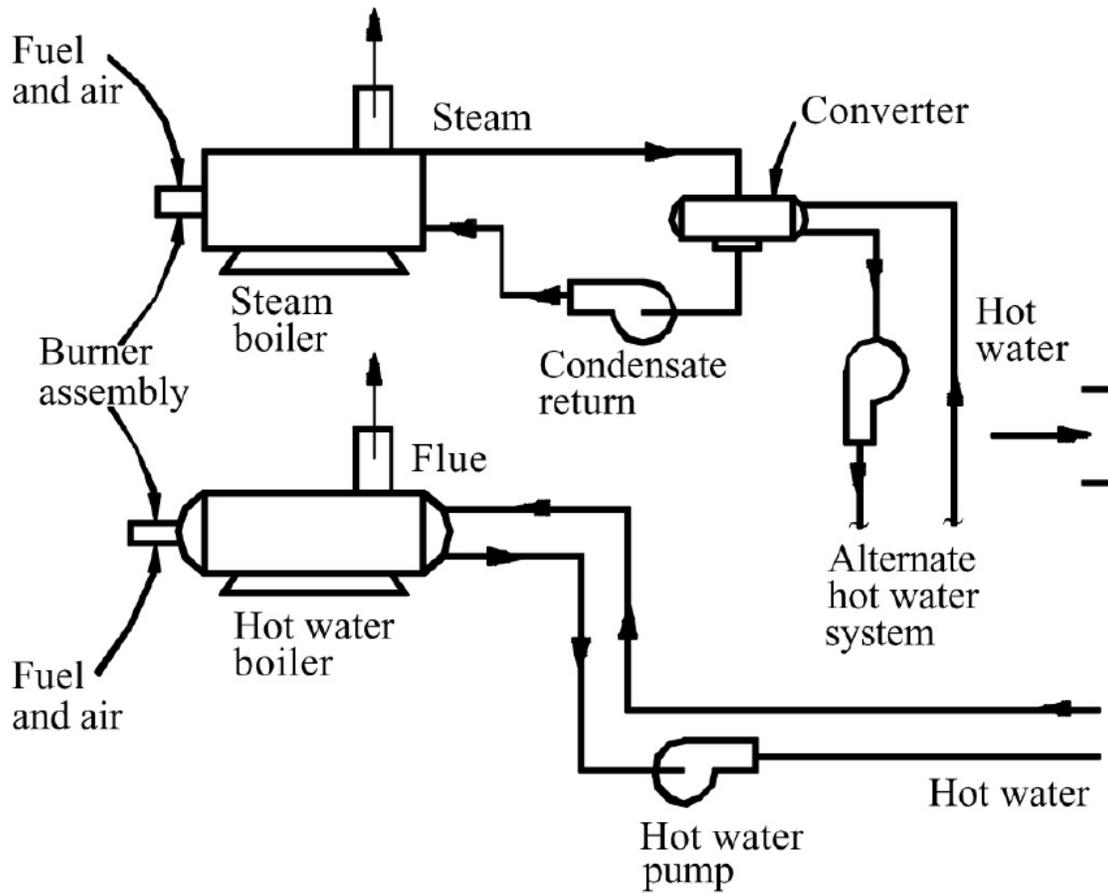
Fig. 1: Figure 7-1. Steam and Hot Water Boilers
