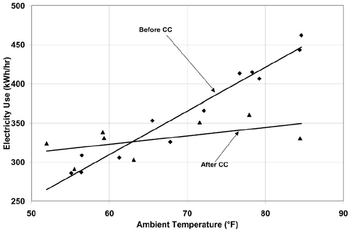
Fig. 4: Figure 4-4. Measured Monthly Average Hourly Whole Building Electricity Consumption Versus the Monthly Average Ambient Temperature
