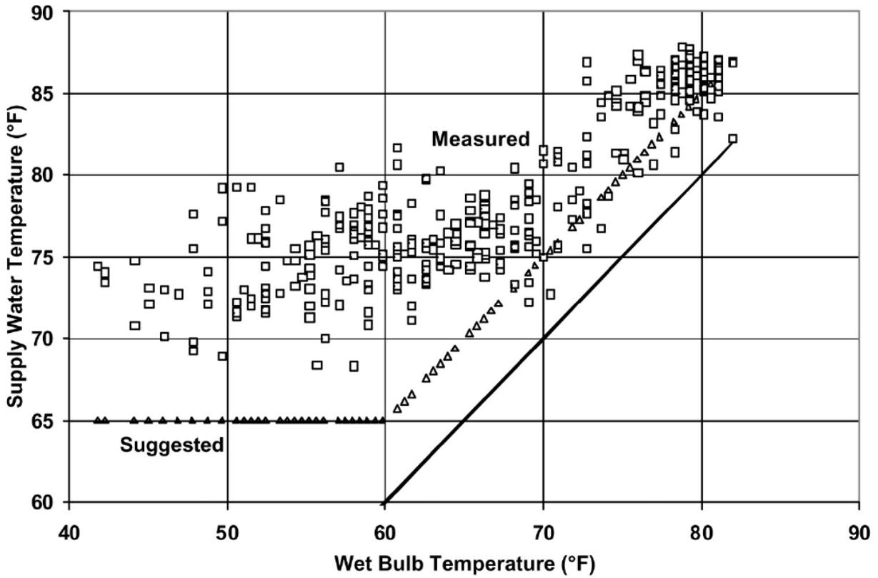
Fig. 2: Figure 6-2. Measured Condenser Supply Water Temperature at the UTMB Chiller Plant as a Function of Ambient Wet Bulb Temperature
