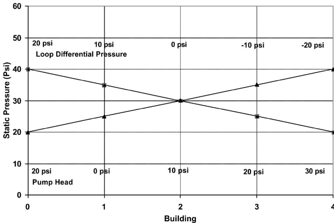
Fig. 6: Figure 5-6. Differential Pressure Distribution for the Evaluation of Combined Source and Distributed Pumping
