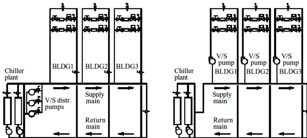
Fig. 1: Figure 5-1. Schematic Diagrams of Source Distributed Pumping (on left) and Distributed Pumping Configurations
