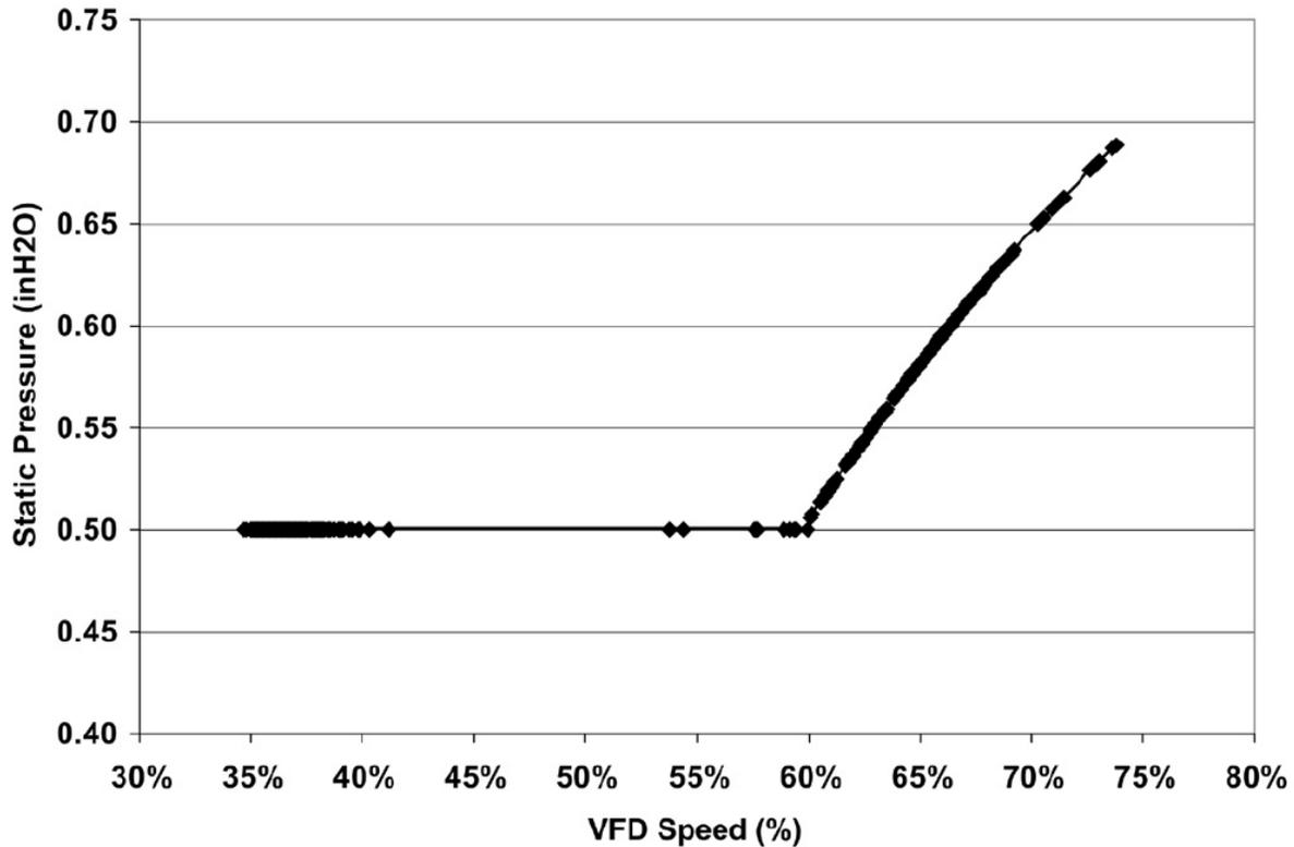
Fig. 6: Figure 4-6. Optimal Static Pressure Reset Schedule and Measured Static Pressure Versus the VFD Speed for AHU-P2 at the CSF Building, M.D. Anderson Cancer Center, Houston, Texas
