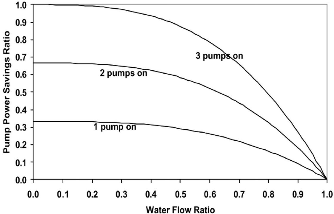
Fig. 5: Figure 6-5. Potential Primary Pump Power Savings Ratio Versus Chilled Water Flow Ratio through Each Chiller
