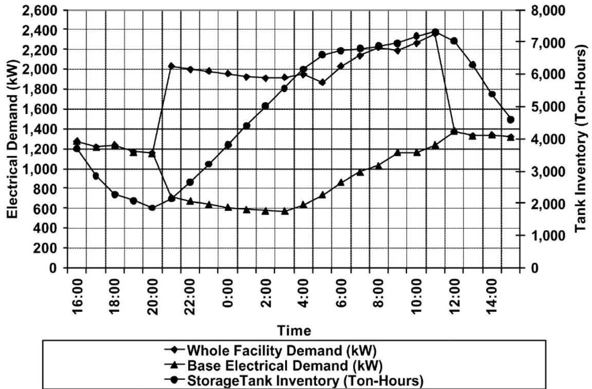
Fig. 9: Figure 8-9. Typical On-Peak Months Whole Facility Demand, Base Electrical Demand and Storage Tank Inventory Profiles
