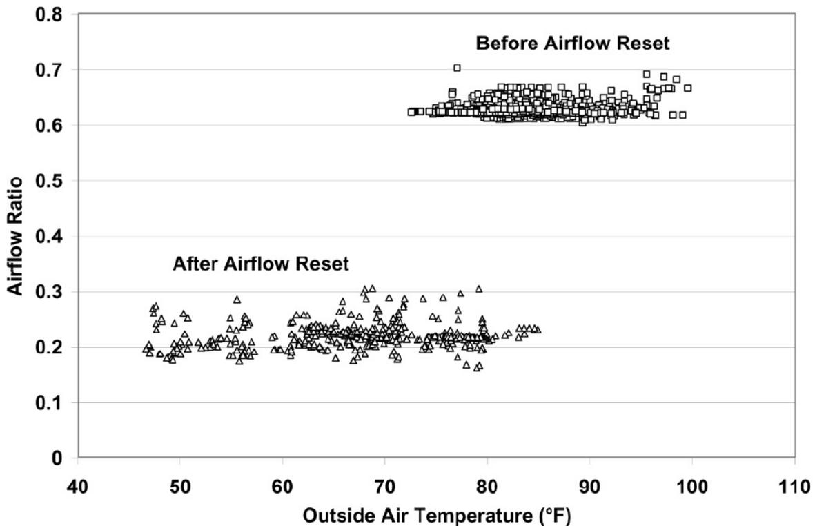
Fig. 25: Figure 4-25. Comparison of Air Flow Before and After Airflow Reset During Unoccupied Hours (Airflow Ratio is defined as the ratio of the air flow to the design air flow)
