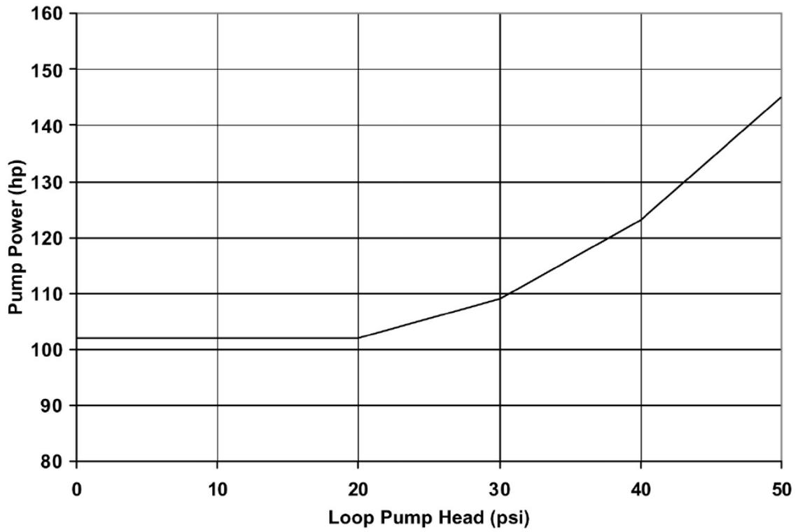
Fig. 7: Figure 5-7. Pumping Power as a Function of Loop Pump Head for the System Considered in the Example
