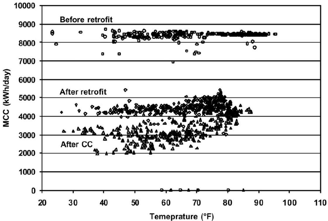
Fig. 5: Figure A-5. ZEC Daily Motor Control Center Electricity Consumption for 1990 Before the Retrofit, 1994 After the Retrofit and 1997 After CCSM
