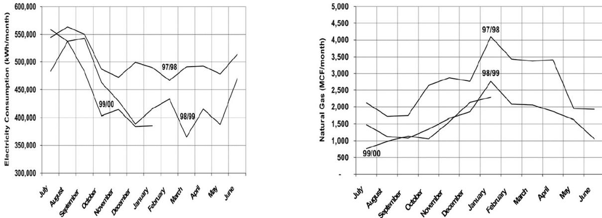
Fig. 3: Figure 4-3. Natural Gas and Electricity Consumption at the Materials Research Institute Before and After Implementation of CCSM Measures
