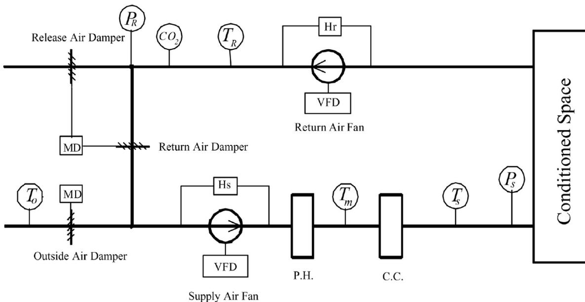
Fig. 21: Figure 4-21. Airflow Control Schematic of the VSDVT Method
