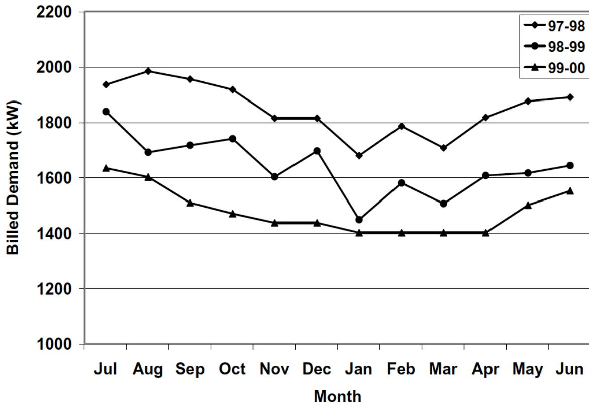
Fig. 11: Figure 8-11. Comparison of Billed Electrical Demand Before and After Commissioning
