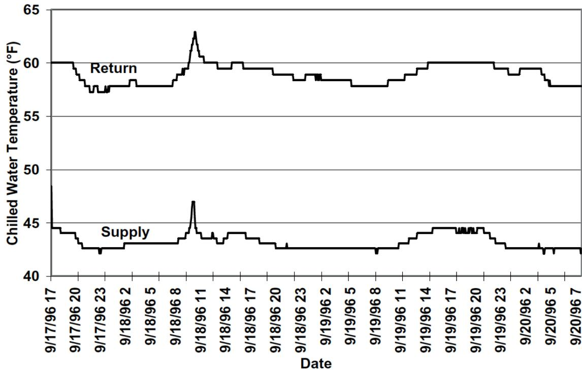
Fig. 4: Figure 6-4. Measured Chilled Water Supply and Return Water Temperature After Building Commissioning (the building differential temperature was less than 10°F before commissioning)
