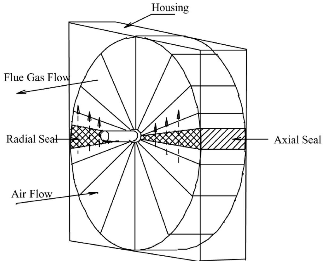
Fig. 5: Figure 7-5. Schematic of Regenerative Air Preheater
