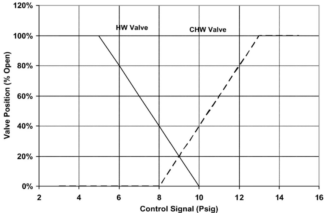
Fig. 12: Figure 4-12. Typical Valve Overlap for a Coupled Control System
