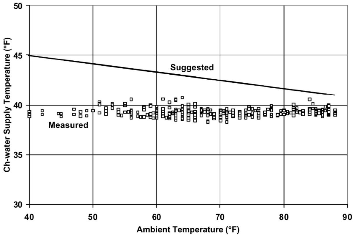
Fig. 3: Figure 6-3. Measured And Suggested Chilled Water Supply Temperature at UTMB
