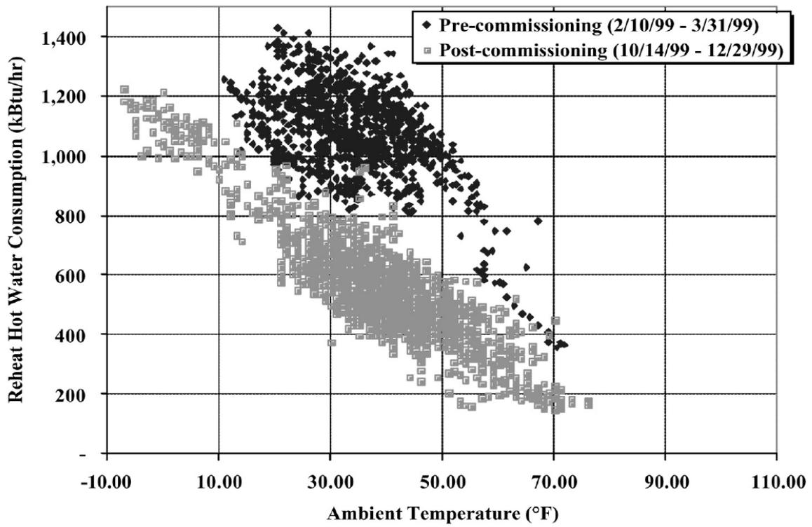
Fig. 3: Figure 2-3. Hourly Reheat Energy at Riverside North (15-minute data)
