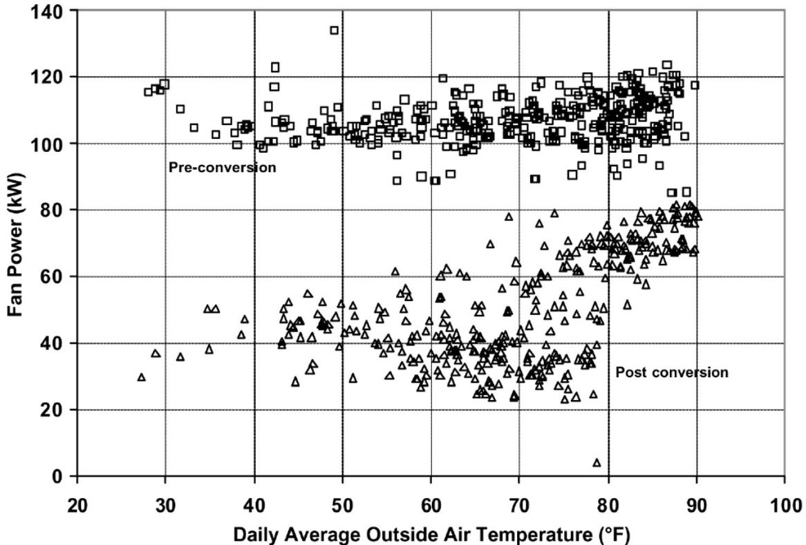
Fig. 16: Figure 4-16. Measured Fan Power Before and After Implementing the CCSM Measures
