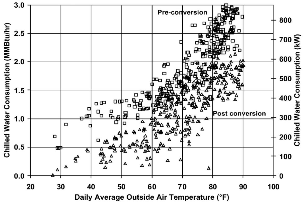
Fig. 17: Figure 4-17. Measured Chilled Water Consumption Versus the Daily Average Outside Air Temperature
