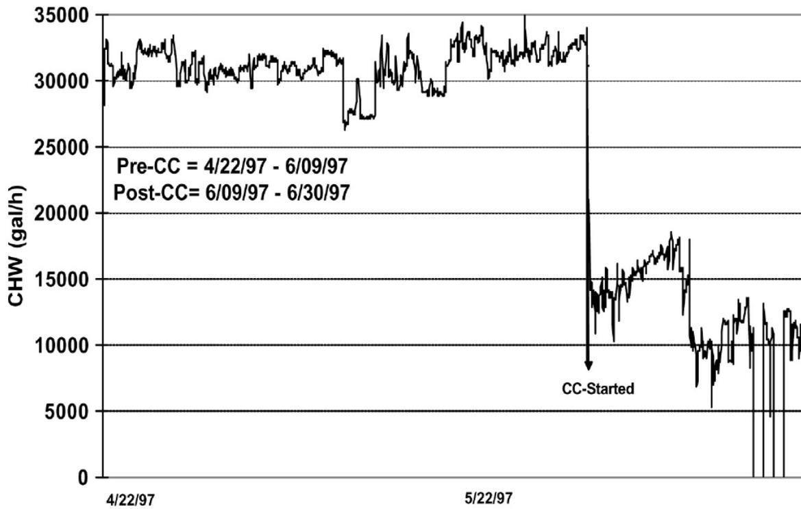
Fig. 2: Figure 5-2. Comparison of Measured Chilled Water Flow Under Both Initial and Optimal Differential Pressure Reset Schedules
