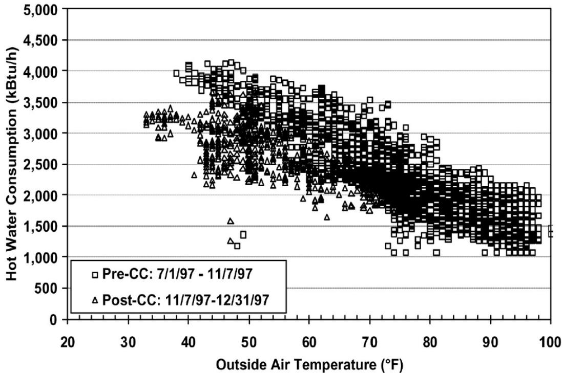
Fig. 14: Figure 4-14. Comparison of Hot Water Energy Consumption Before and After Implementation of CCSM Measures
