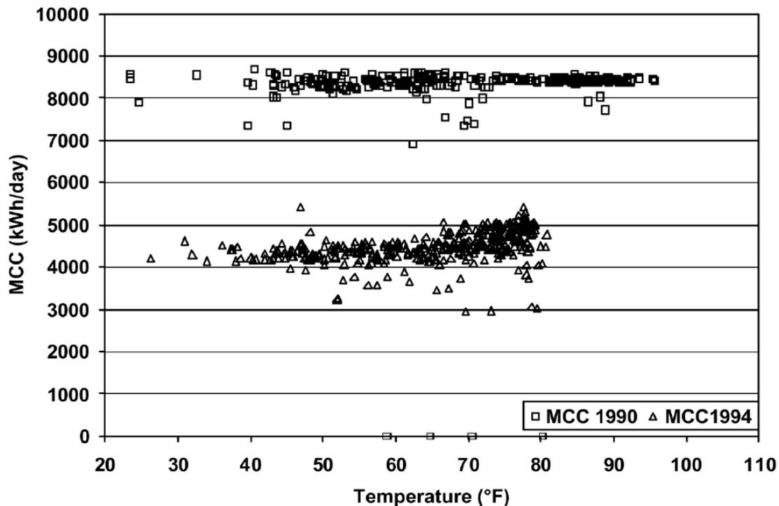
Fig. 2: Figure A-2. ZEC Daily MCC Consumption in 1990 Before the Retrofit, in 1994 After the Retrofit
