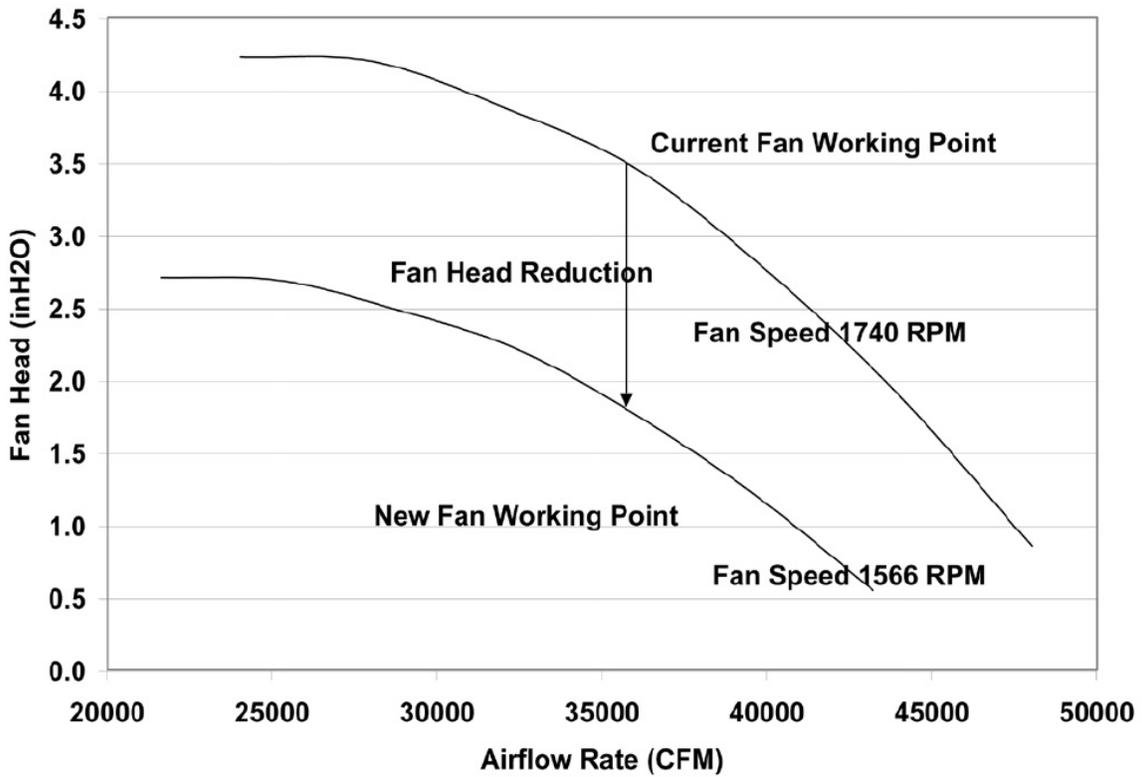
Fig. 1: Figure 4-1. Determining New Fan Speed Using Measured Fan Head Reduction and Fan Performance Curve
