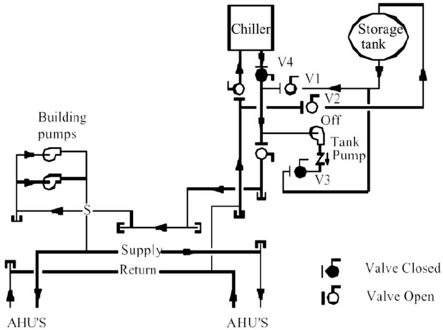
Fig. 3: Figure 8-3. Waterside Schematic of the Chiller/Thermal Storage System at the Hospital in Monahans, Texas
