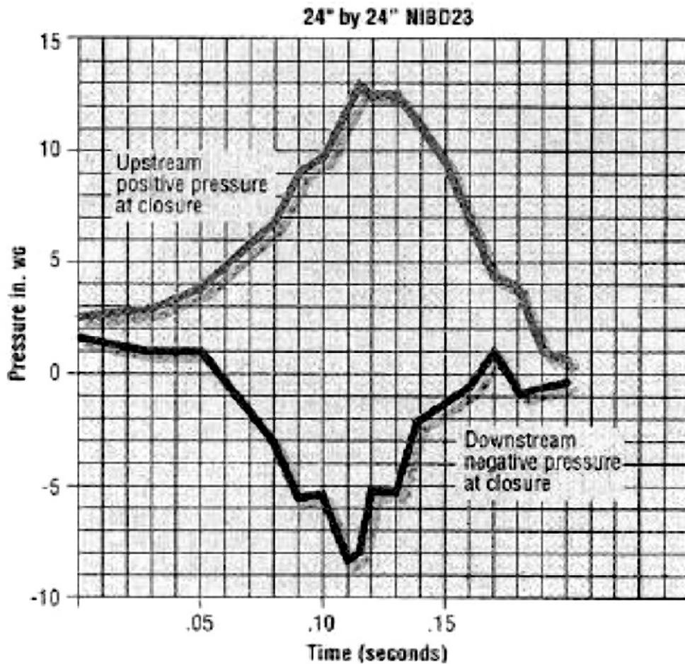
Fig. 15: Figure 4-15. Static Pressure Versus Time Upstream and Downstream of a Fire Damper When Suddenly Closed
