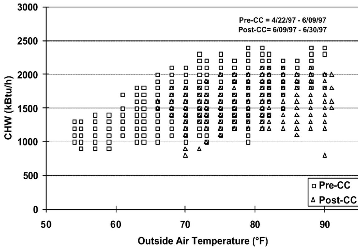
Fig. 3: Figure 5-3. Comparison of Chilled Water Energy Consumption Under Original and Optimal Chilled Water Differential Pressure Schedules
