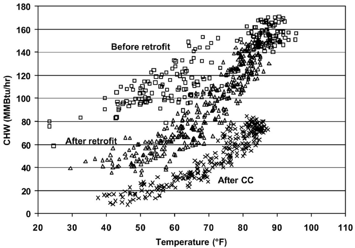
Fig. 6: Figure A-6. ZEC Daily Chilled Water Consumption for 1990 Before the Retrofit, 1994 After the Retrofit and 1997 After CCSM
