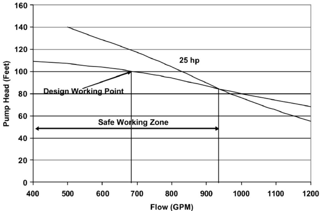
Fig. 10: Figure 5-10. Chilled Water Pump Curve (regenerated using pump curves from TACO, TA Series Model 1229, speed 1760 RPM, and 10.25” impeller)
