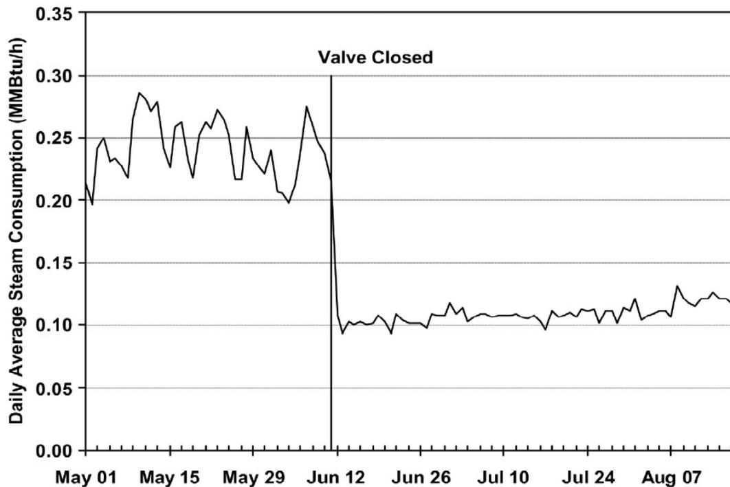
Fig. 1: Figure 3-1 Comparison of Measured Daily Average Steam Consumption Before and After Manually Shutting Off Heating Coil Valves in the Business Administration Building at University of Texas at Austin
