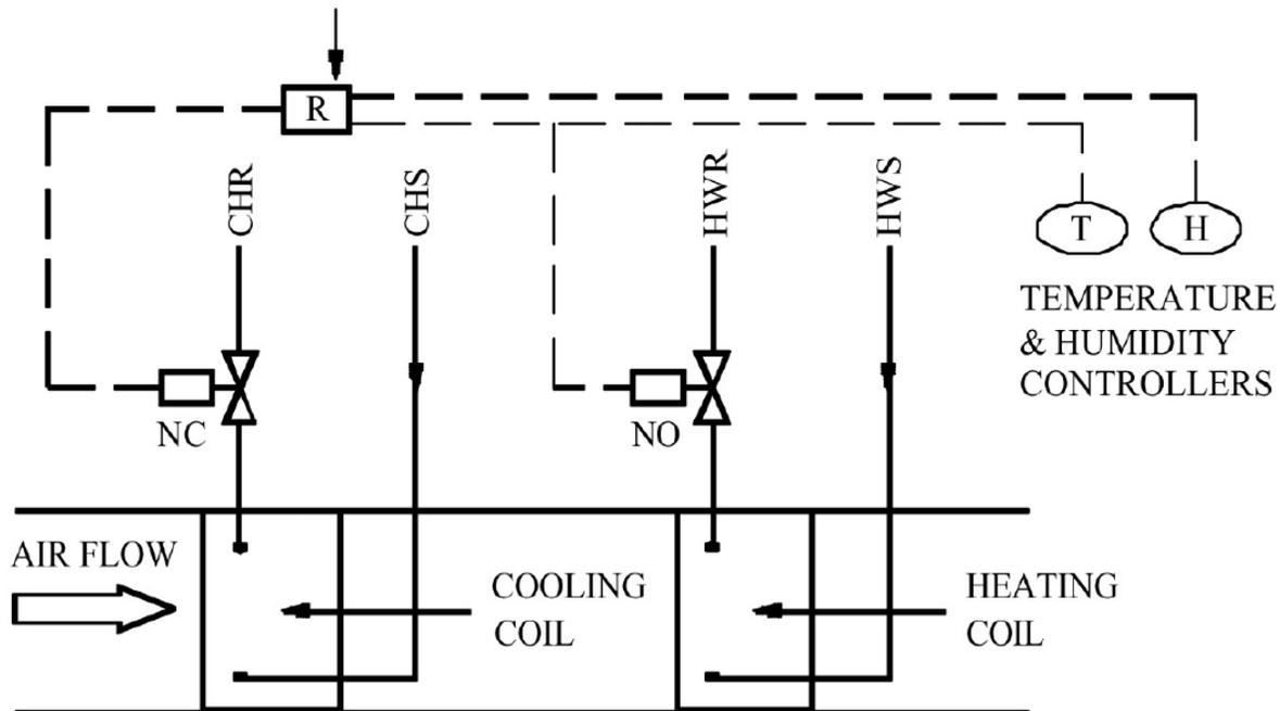
Fig. 11: Figure 4-11. Schematic Diagram of a Coupled Control System
