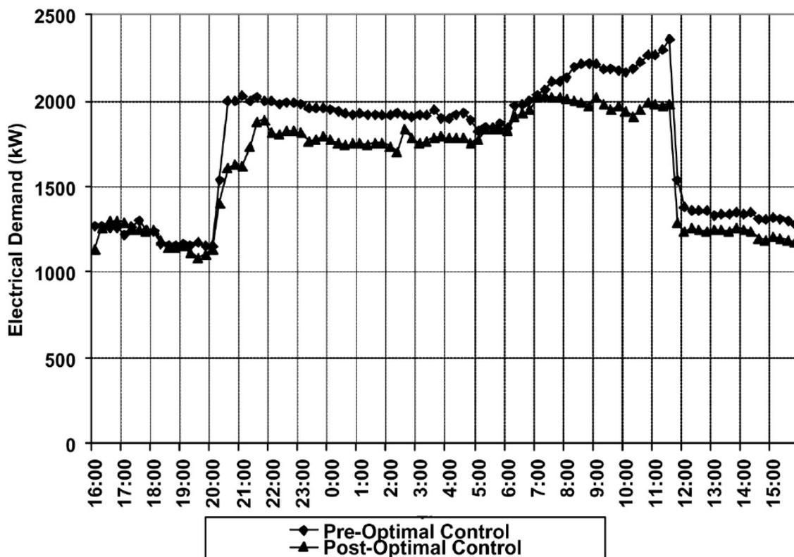
Fig. 10: Figure 8-10. Comparison of Typical Facility Electrical Demand Profile Before and After Implementation of Optimal Control Sequences
