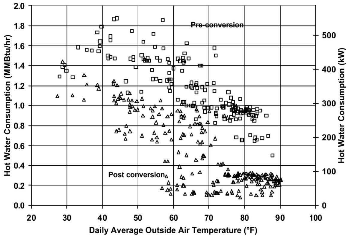
Fig. 18: Figure 4-18. Measured Hot Water Consumption Versus the Daily Average Outside Air Temperature
