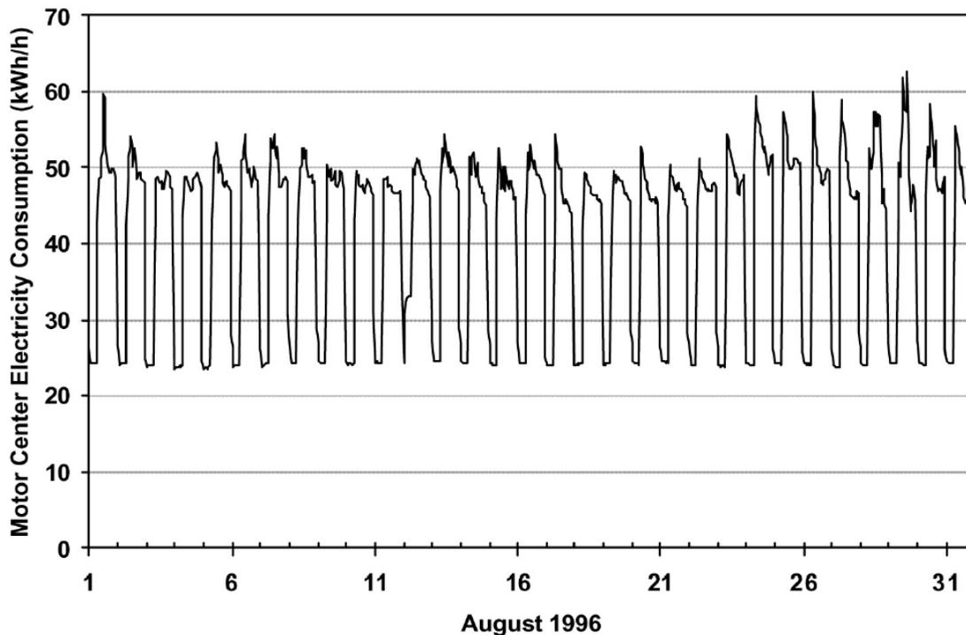
Fig. 3: Figure 3-3. Measured (Post-CC<sup>SM</sup>) Hourly Supply Fan Electricity Consumption in the Education Building
