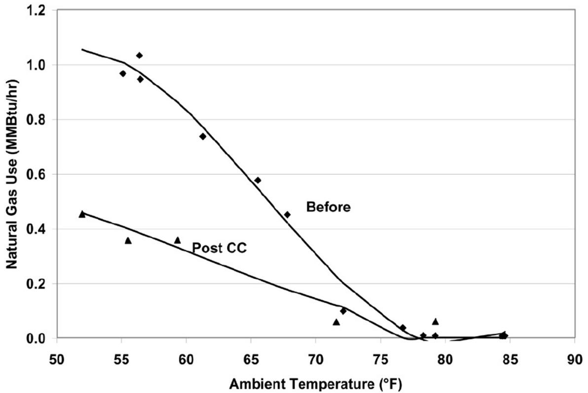
Fig. 5: Figure 4-5. Measured Heating Energy Consumption Versus the Monthly Average Hourly Ambient Temperature
