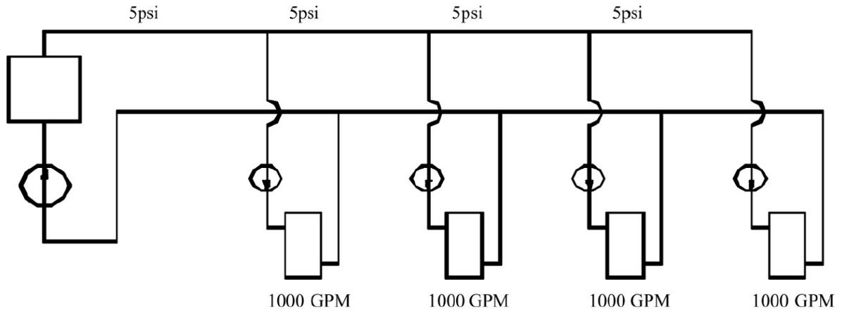
Fig. 4: Figure 5-4. Loop and Building Flows and Pressure Drops for Example Problem
