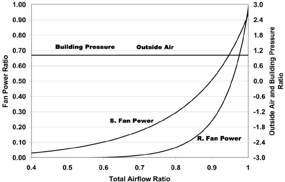
Fig. 23: Figure 4-23. Simulated Building Pressure, Outside Air Intake and Fan Power Using VSDVT Control
