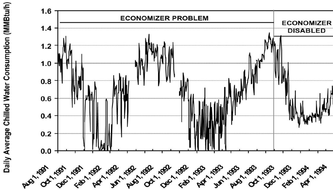
Fig. 10: Figure 4-10. Measured Hourly Cooling Energy Consumption of the Nursing Building in Austin Texas
