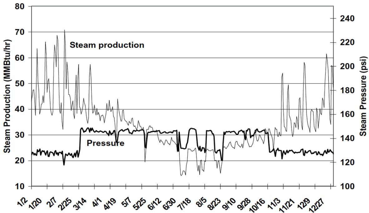
Fig. 3: Figure 7-3. Variation of Steam Consumption and Boiler Pressure with Time at UTMB
