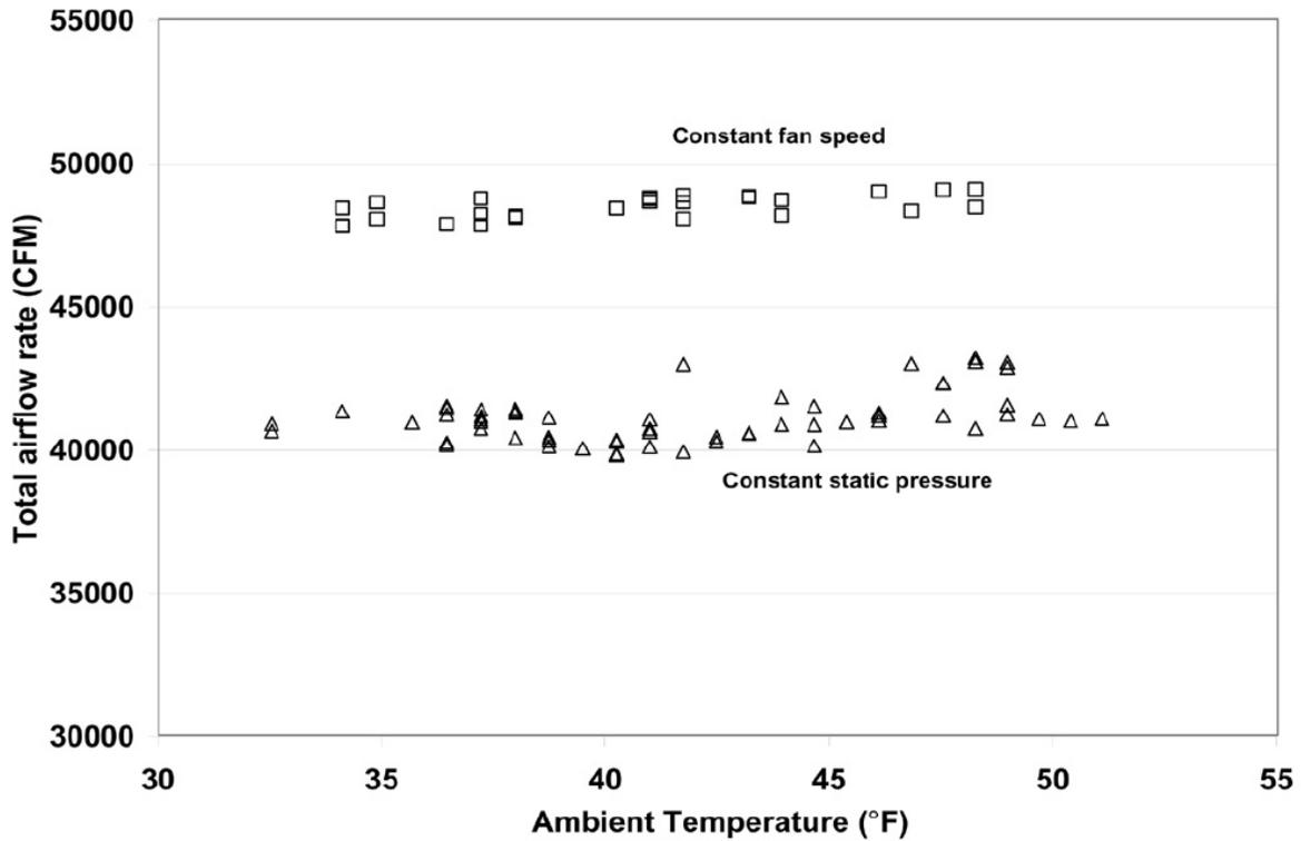
Fig. 19: Figure 4-19. Measured Hourly Total Air Flow for Both the CSFS and the VSFS Operations
