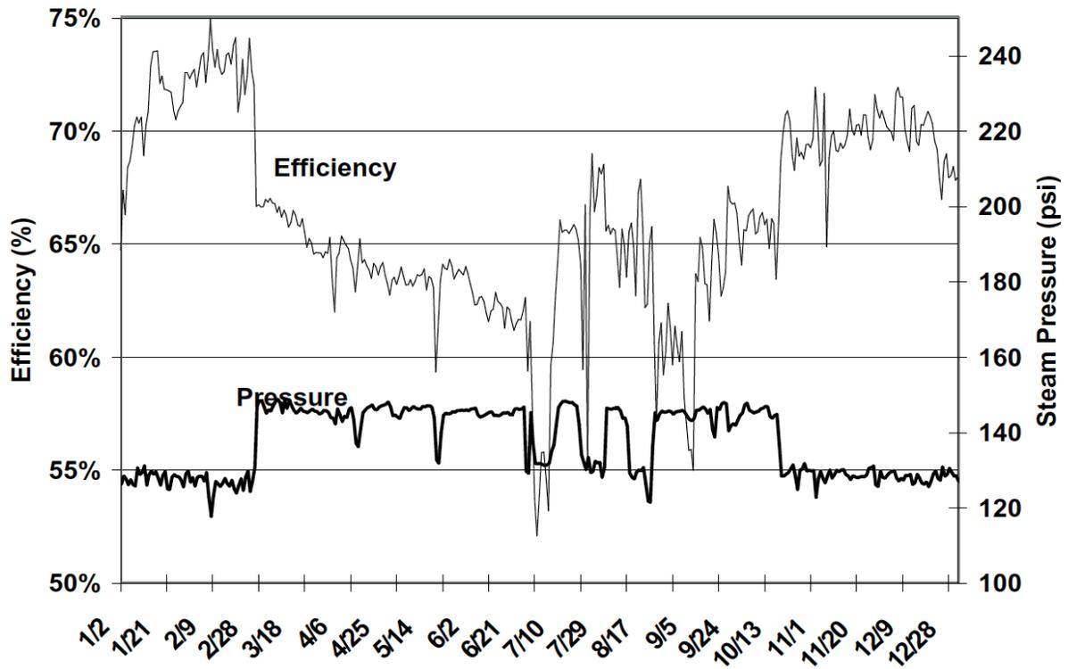
Fig. 2: Figure 7-2. Boiler Efficiency and Steam Pressure at the UTMB Galveston Boiler Plant
