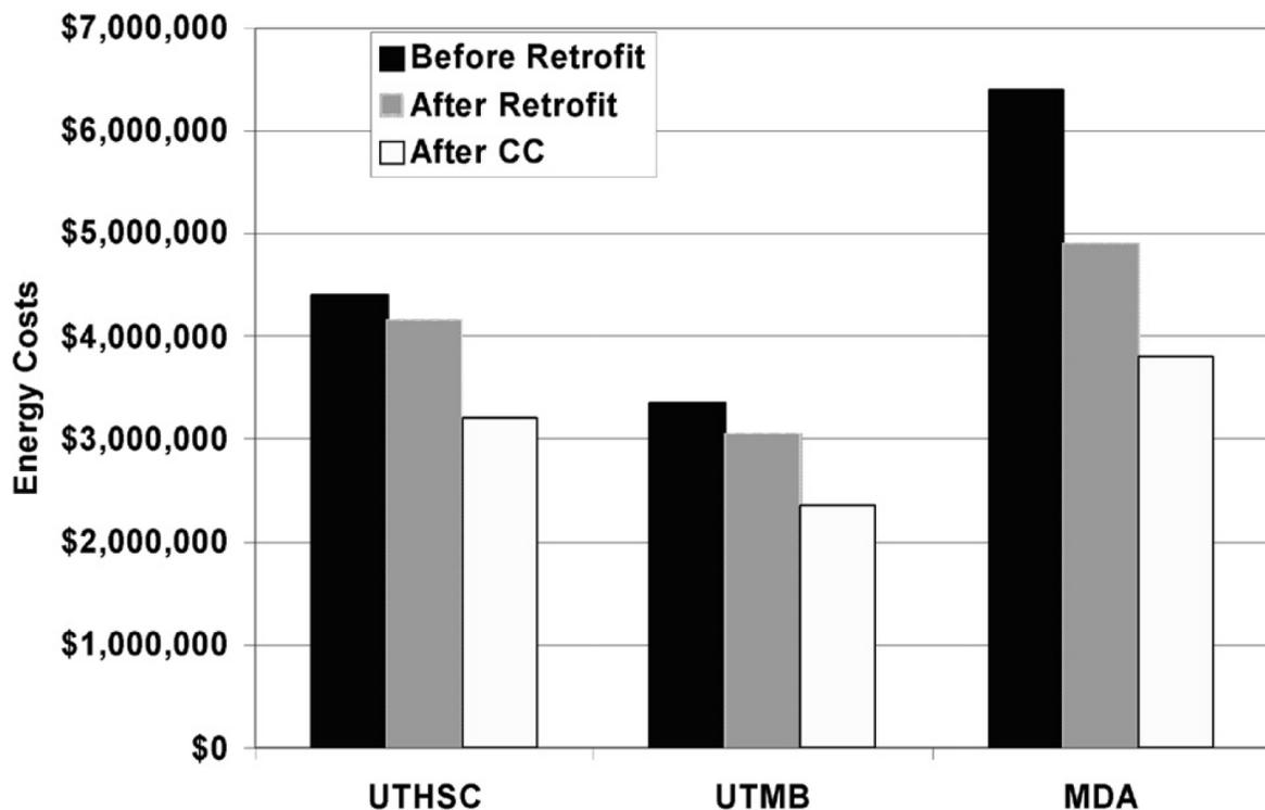
Fig. 1: Figure 2-1. Energy Costs Before Retrofit, After Retrofit, and After Retrofit and CC<sup>SM</sup> at University of Texas, Health Science Center (UTHSC), University of Texas Medical Branch at Galveston (UTMB), University of Texas, M. D. Anderson Cancer Center (MDA)
