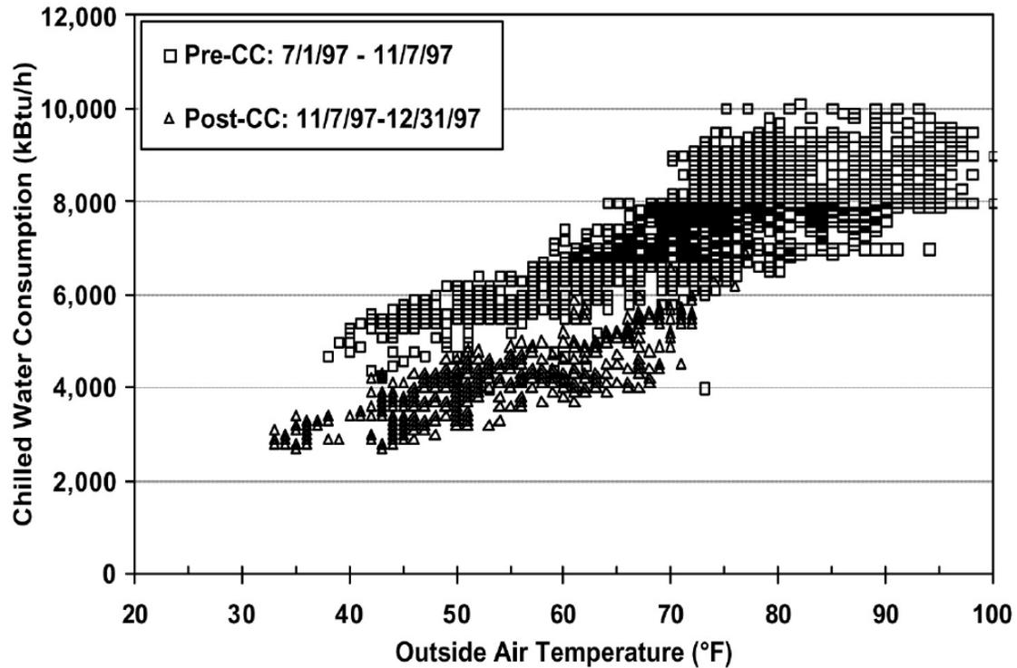
Fig. 13: Figure 4-13. Comparison of Chilled Water Energy Consumption Before and After Implementation of CCSM Measures
