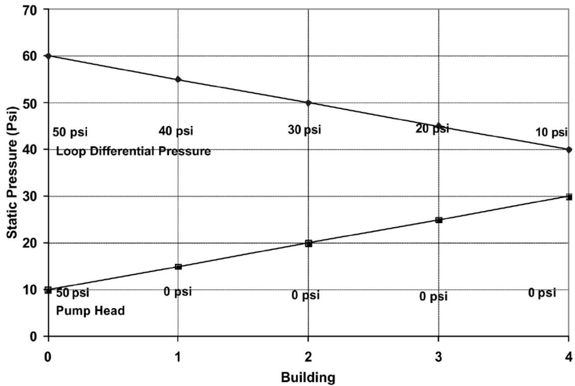
Fig. 5: Figure 5-5. Differential Pressure Distribution for Source Distributed Pumping
