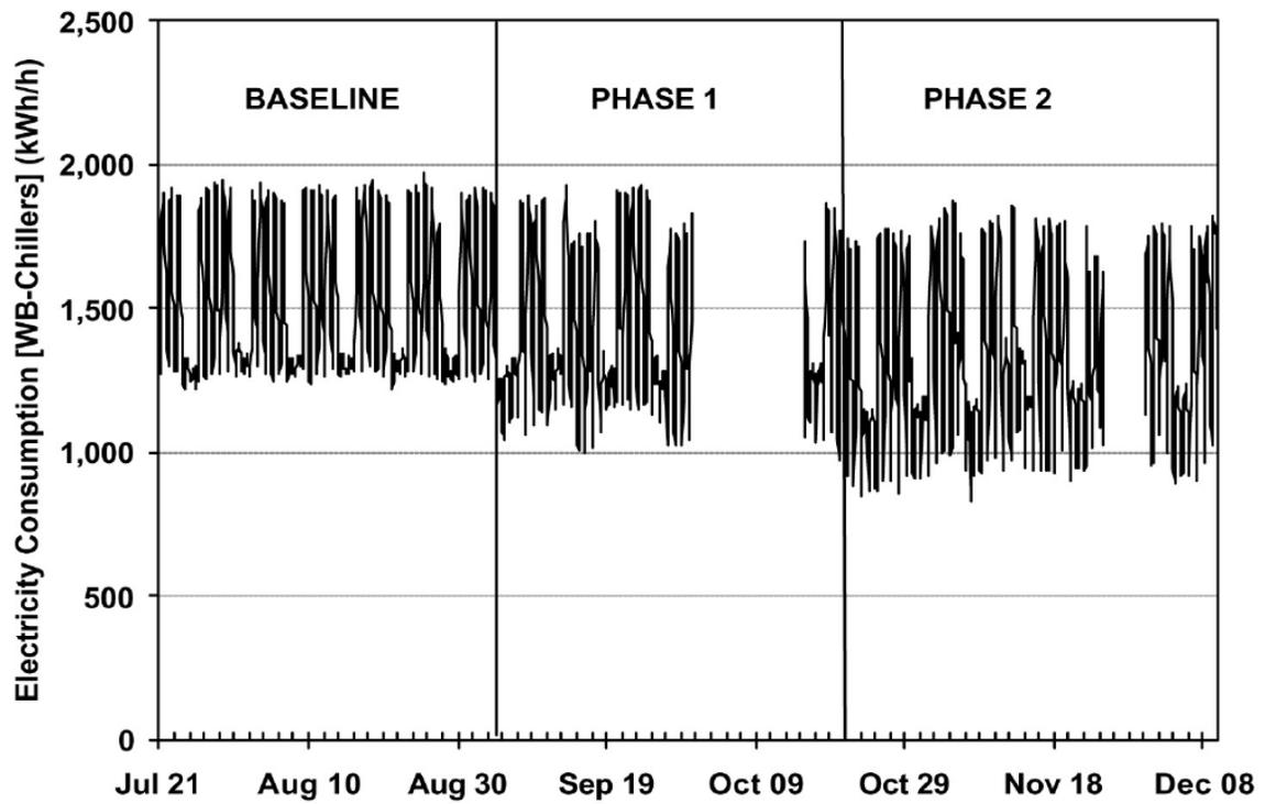
Fig. 2: Figure 3-2. Hourly Whole Building Electricity Consumption at the Stephen F. Austin (SFA) Building Before and After Night Shut Down of AHUs Was Initiated
